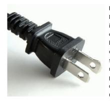
Electrical Polarized Plug: This Cut + Dry Dehydrator has a polarized plug (one blade is wider than the other). To reduce the risk of electrical shock, the plug is intended to be used by inserting it into the electrical outlet only one way. If the plug does not fit securely into the outlet, turn the plug and re-insert. Do not modify this plug. If the plug does not fit the outlet securely, call a qualified electrician for assistance. DO NOT use this plug with extension cords of any kind.
